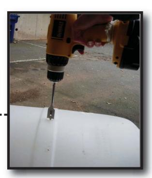
Step. 3: Using the 13/16" drill bit again, drill an opening for the stopper at the very bottom edge of the barrel.
